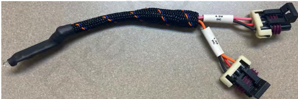
On a LiquiShift system, plug the Pressure Simulator into the Control Pressure connector.
