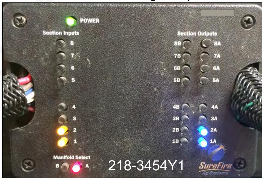
**Section OUTPUTS (BLUE)** to section valves are on right (to 23-pin connector to valves)
