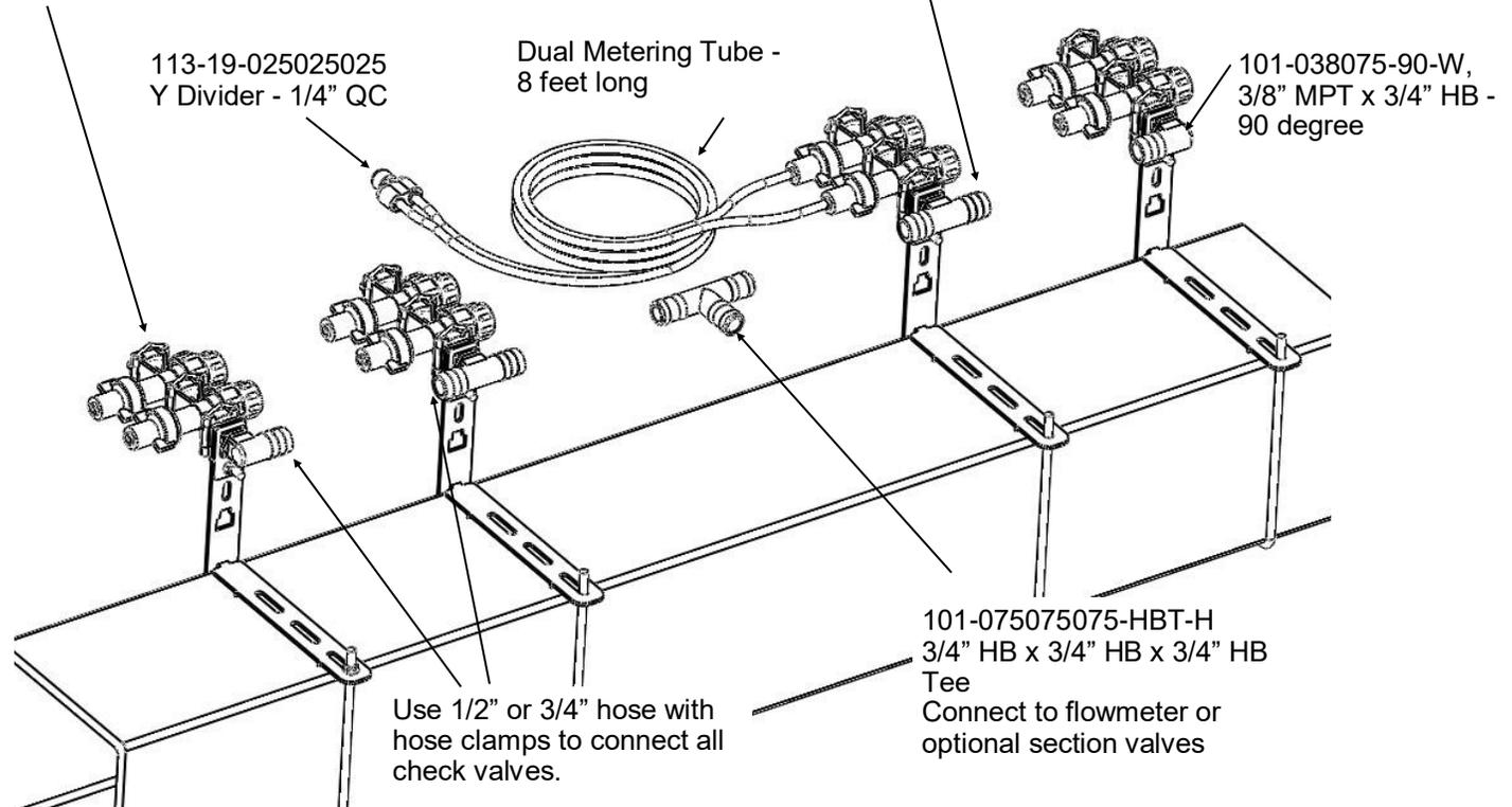
This is a general diagram showing the dual check valve assembly mounted on a planter toolbar. The check valve and bracket are very flexible in their mounting. The check valve can mount behind, directly over, or in front of the toolbar. The check valve can be put in the bracket facing up & down or sideways (shown). In addition, the steel bracket could be rotated 90 degrees and clamp around the bar. The multiple slots in the bracket are used to mount to any tube 7x7 inches or smaller.
