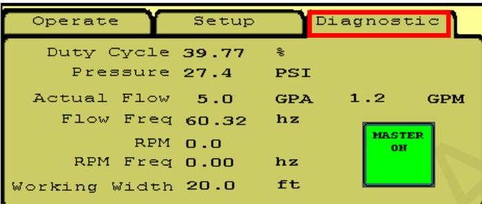
**Diagnostic Tip:** Note the relationship between Duty Cycle (%), Pressure, Flow (GPM), and RPM (hydraulic pump). If Duty Cycle and RPM increase above what is normal for a given flow, there could be a restriction on the inlet side of the pump. This could be a plugged strainer or a strainer that gets gelled over, especially with cold fertilizer. Increased Duty Cycle with no increase in RPM could mean the pump is not getting enough hydraulic flow to spin the pump faster.
