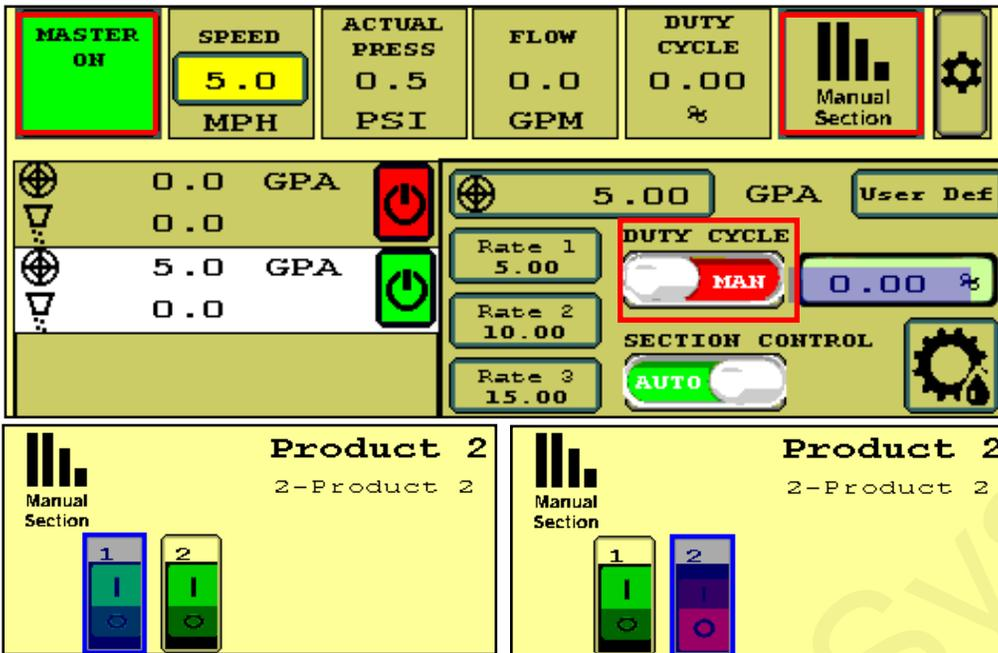
To operate the Section Valves manually, press **Manual Section**, then press any section button to turn the valve off/on.
