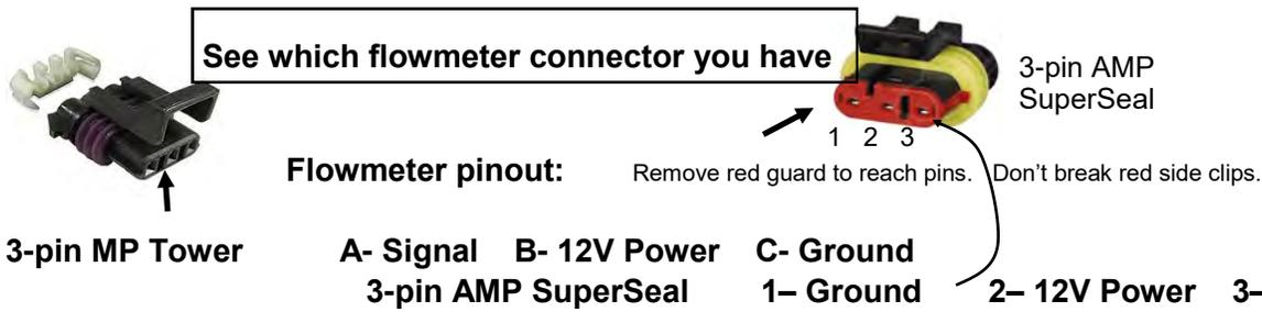
1. Unplug the flowmeter. With voltmeter, check for **12-13 volts between Power & Ground** of flowmeter connector. Should have **4-5 volts** (may have 9 v) **between signal and ground**. If voltage is not present, inspect wiring harness and check for voltage at harness connection(s) nearer the Rate Controller.
