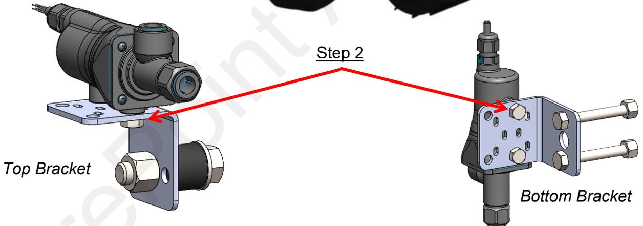
3. Use the provided u-bolts to secure the hose to the mounting bracket.
