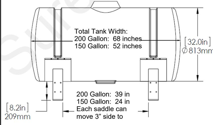
Saddle footprint with bolt holes. 3/4" slots fit from 6" to 8" wide tube directly.
