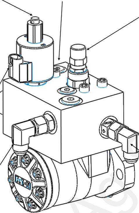
**Bypass Valve**—Remove the cap to access a bypass needle valve. This valve is shipped from the factory closed. **The only case when valve should be open is when running in series with other hydraulic motors.**
