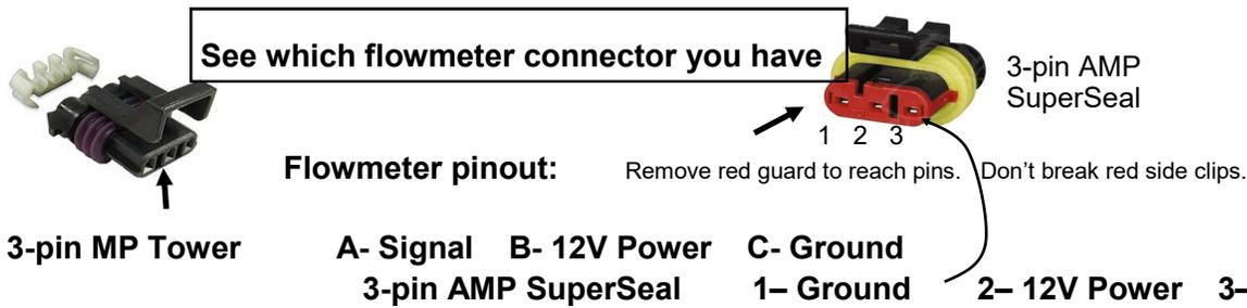
1. Unplug the flowmeter. With voltmeter, check for **12 volts between Power & Ground** of flowmeter connector. Should have **4-5 volts between signal and ground**. If voltage is not present, inspect wiring harness and check for voltage at harness connection(s) nearer the Rate Controller.
