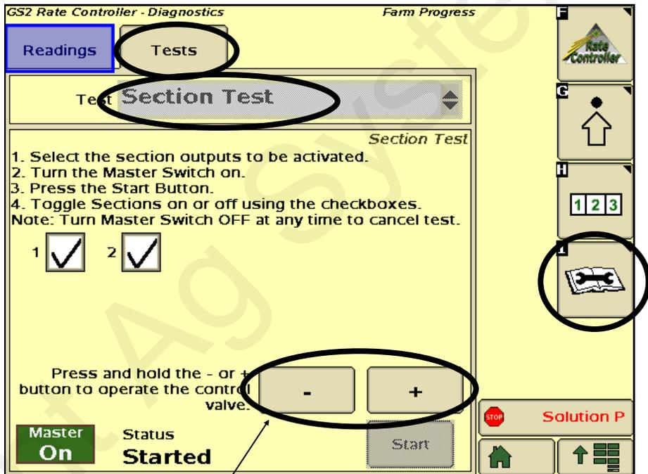
9. **Make sure the GS2 or GS3 flow readout in GPM can be increased and decreased with the plus & minus buttons.**
