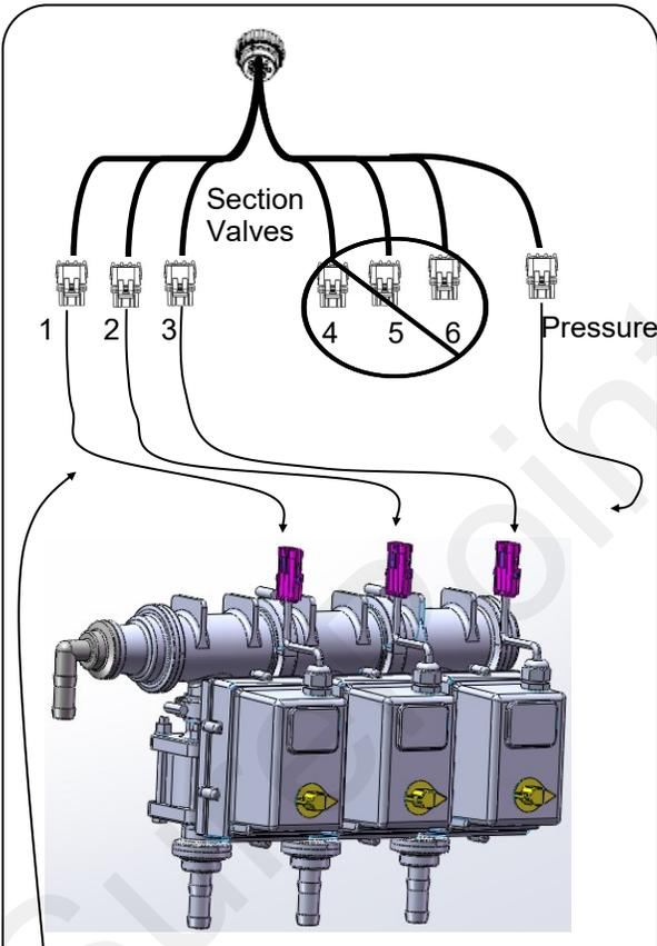
Can use 3-Pin Weatherpack Extension cables to reach section valves
