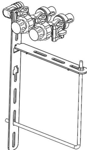
**Example 3.** Use the long bracket on the front of a 3x7 bar (vacuum tube on some planters). Mount the check valve hanging forward of the bar. The supply line will run directly over the bar. The excess bolt and bracket length can be cut off.
