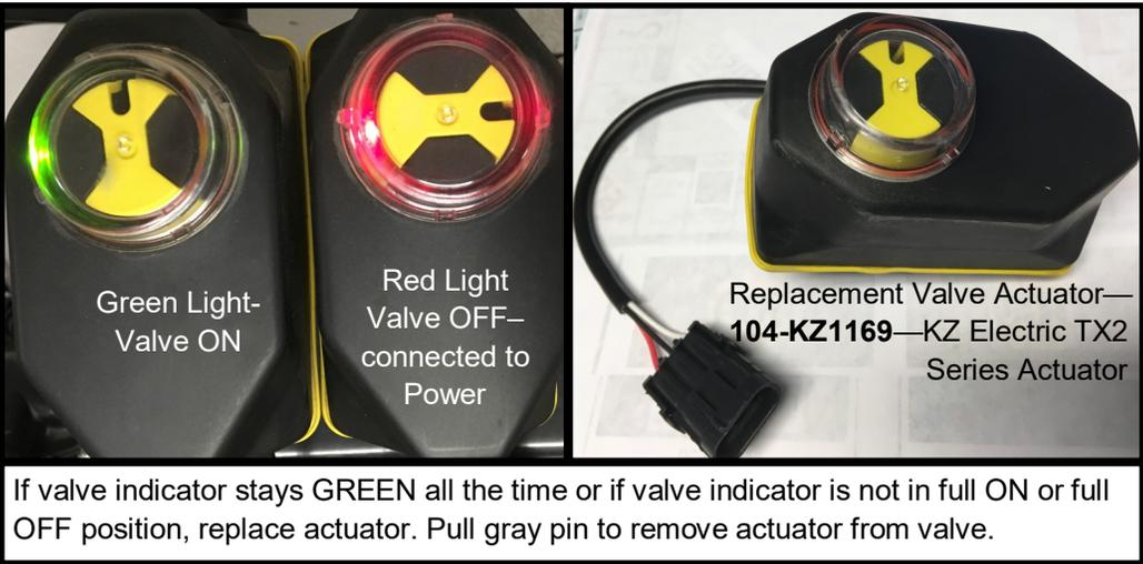
**This is a 3-way valve.** If product will not flow when valve is ON, either move the outlet hose to the other port, or remove actuator and rotate valve ball 180°, and replace actuator.
