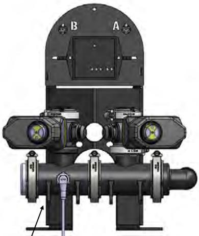
Pressure Sensor for LiquiShift is mounted at the base of the valve stack. The same sensor is used for LiquiShift and displayed on the Ag Leader display.
