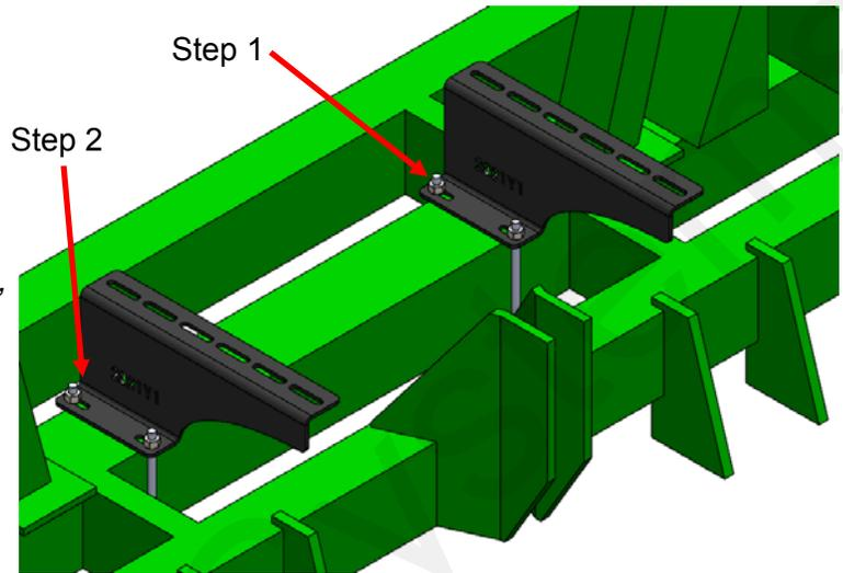
3. Position SureFire Ag Torpedo bracket (PN 2719Y1, Not Included in Kit 516-04-150150) on 2821Y1 brackets. Bolt loosely using 1/2" hex head bolts and 1/2" flange nuts.
