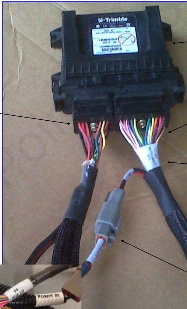
Trimble Field-IQ Rate and Section Control Module
