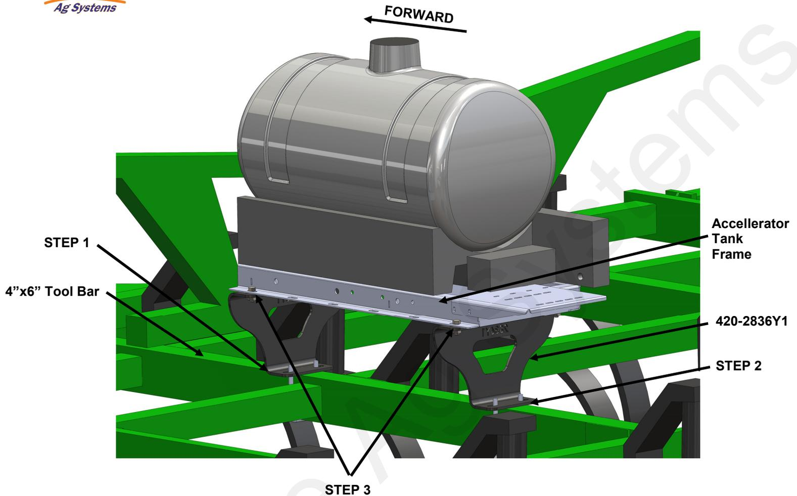
1. Mount the Front Tank Stand (420-2836Y1) as shown in picture above using the provided Square Bend U-bolt (380-1041). Do not tighten to allow for adjustment in Step 3.
