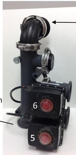
The rinse valve assembly attaches here (inside the cabinet).
