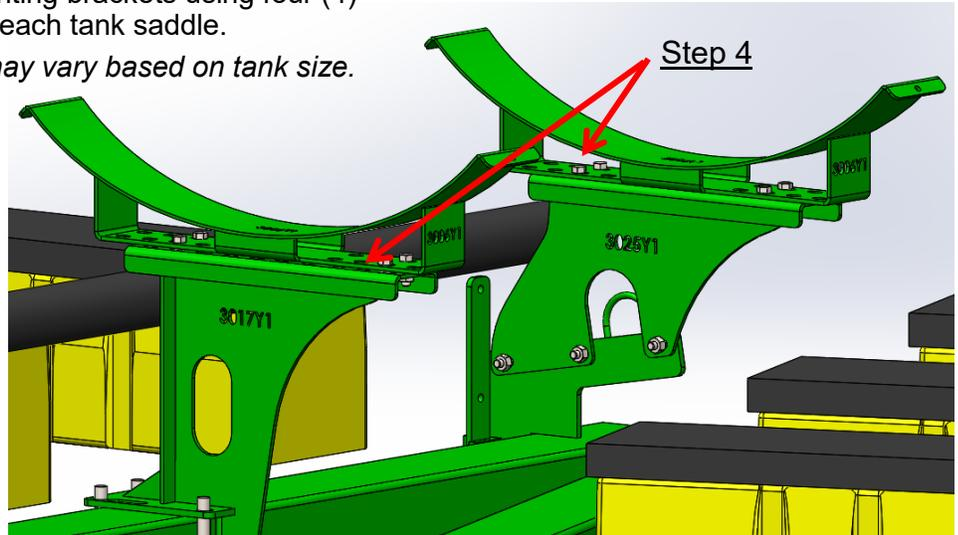
5. Place tank support sheet and tank in saddle. *Note: Part number for tank support sheet may vary based on tank size.*
