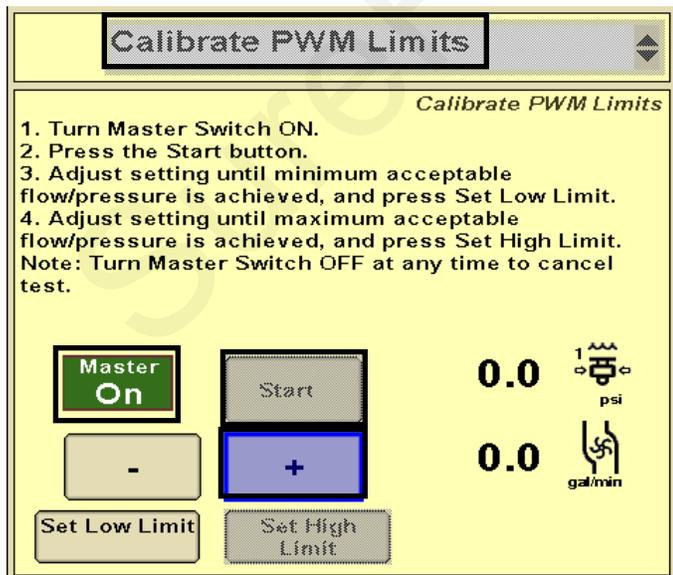
The **Calibrate PWM Limits Test** is a very useful diagnostic tool in servicing the John Deere system. It is a good way to prime the pump initially. It can be helpful to go the **Readings > Delivery System** to see information on the flowmeter operation and the **PWM Duty Cycle**.
